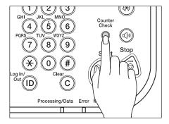
Press [Counter Check] on the control panel.
